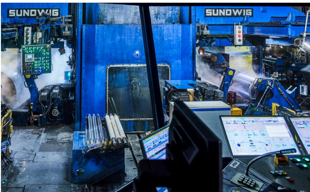
Figure 1. The “Sundwig 1350” 20-high cold rolling mill at the Dillenburg works. The VTLG can be recognised from the light blue indicator light on the mill to the right of the control panel (Picture: Wolfram Schroll / Vollmer GmbH)
